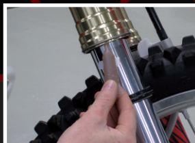
6. Apply grease between inner- and outertube
